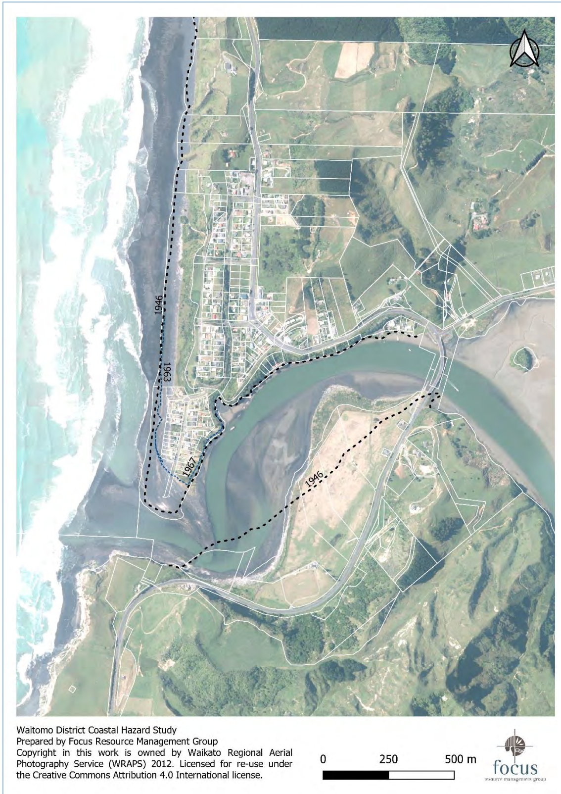
Figure 15: Shoreline change since 1946 at Mokau River entrance. Parcel boundaries provide insight into the original length of Point Road.
