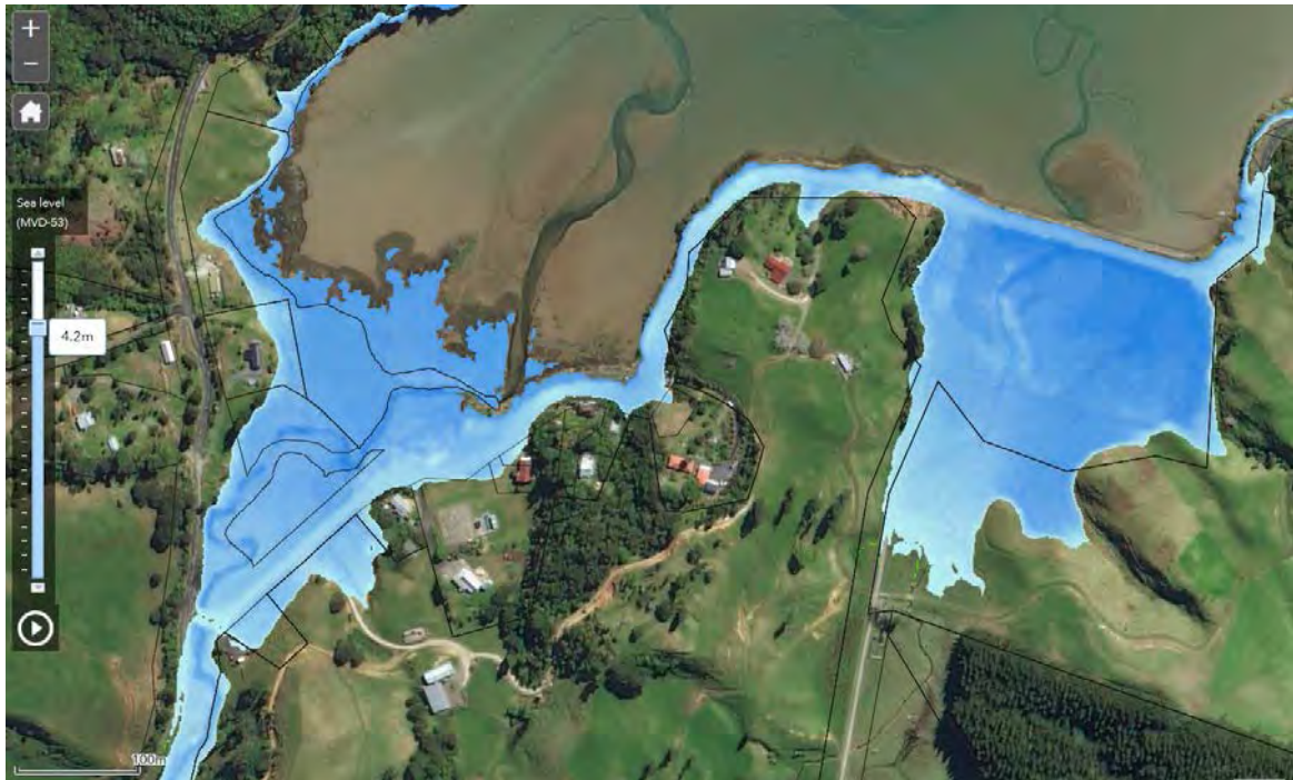
Figure 48: Areas of land (blue) at Kinohaku below the elevation of coastal inundation in an extreme storm surge event with 1.0 m of sea level rise (4.16 m MVD '53). For Discussion of levels see Section 4.2. Green areas indicate land below the elevation of flooding, but with no clear hydraulic link to the coast. Waikato Regional Council Coastal Inundation Tool http://coastalinundation.waikatoregion.govt.nz/ .
