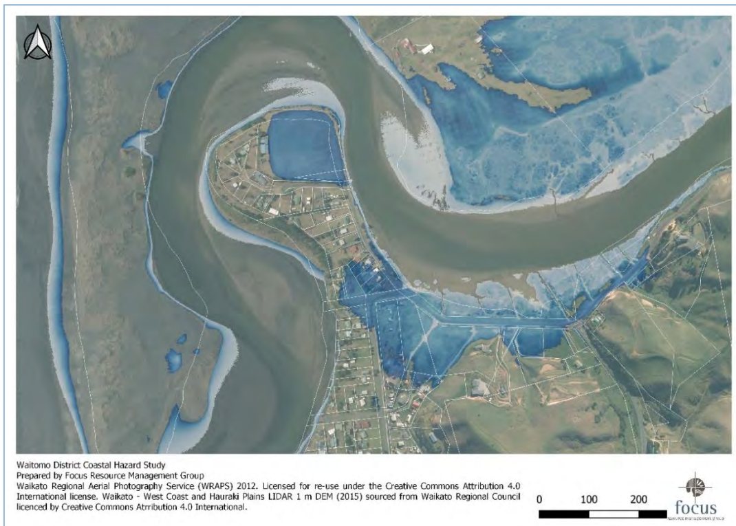
Figure 38: Areas of land below the elevation of coastal inundation in an extreme storm surge event (3.16 m MVD '53). For Discussion of levels see Section 4.2.
