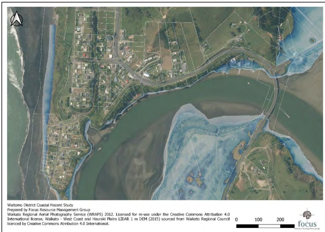
Figure 20: Shoreline between the Mokau township and Mokau River bridge. Blue indicates areas of land below the elevation of a severe storm surge with 1.0 m sea level rise.
